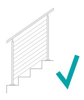
Cables posts will be screwed down on the top of the threads/steps or flat landing.
