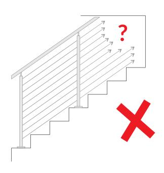
Cables won't have an "end' to be attached to.
